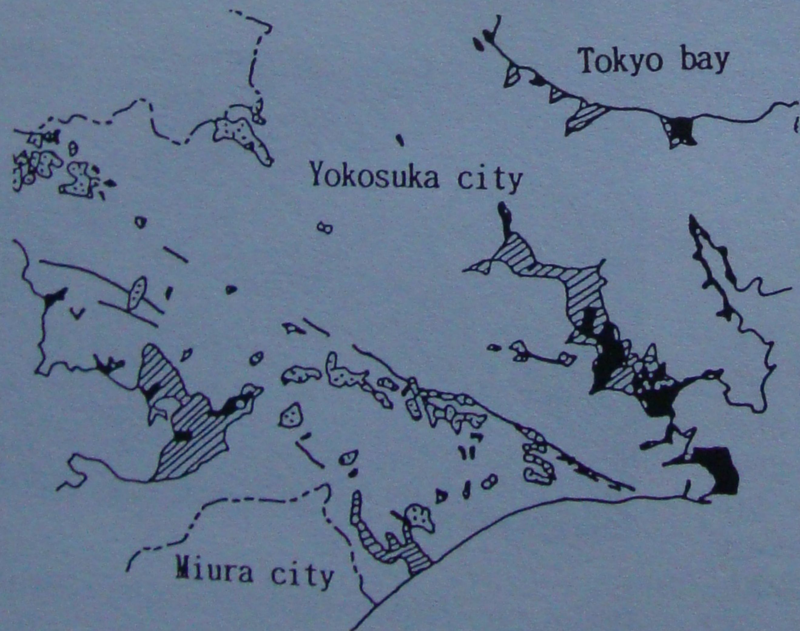
Fig. 3 Zoning in accordance with the classification of seismic risks
